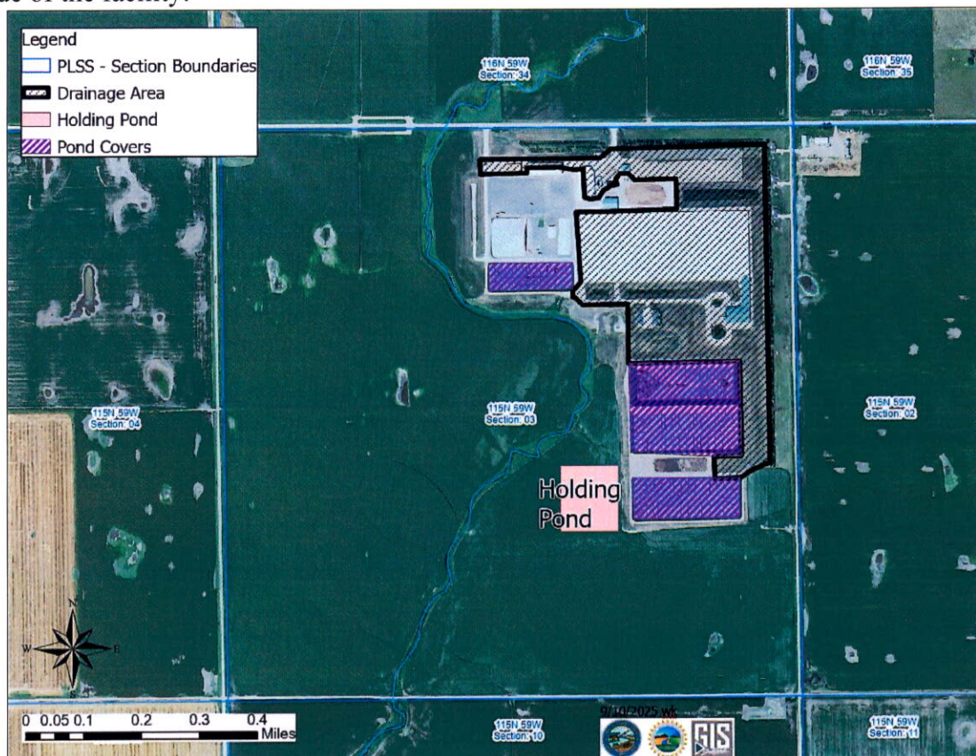
Figure 1: Proposed holding pond location and runoff area
