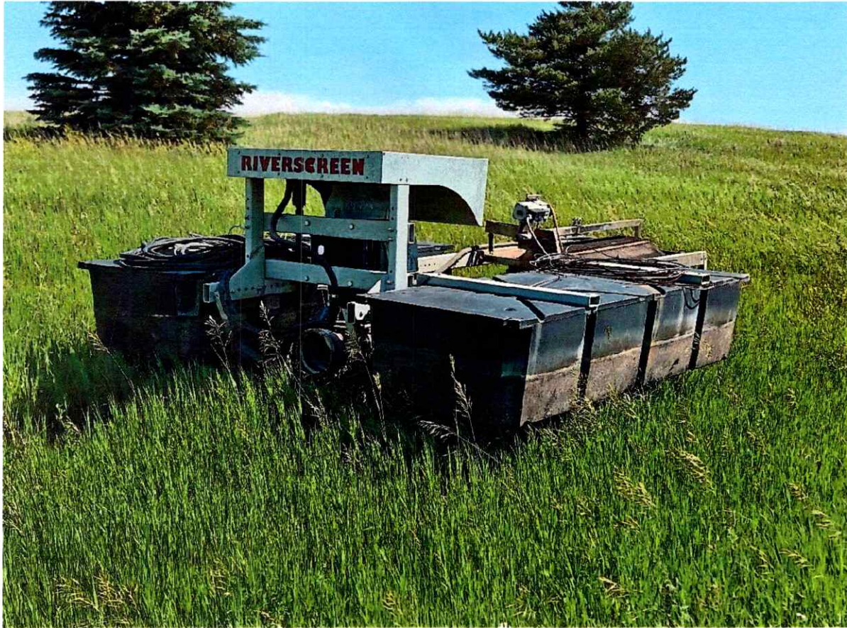
James River floating platform pumping plant.
