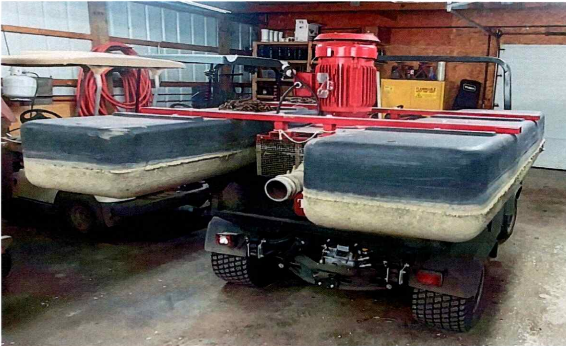
Centrifugal pump powered by a 10 hp electric motor supported by floats that draws water from the Split Rock Creek.
