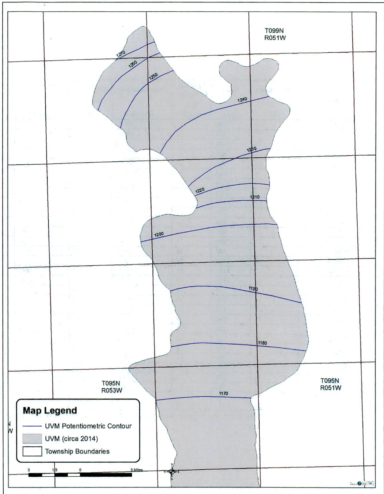
Figure 4. January 21, 2014, potentiometric surface of the main body of Upper Vermillion Missouri aquifer in feet above mean sea level (SD-Geological Survey, in progress)
