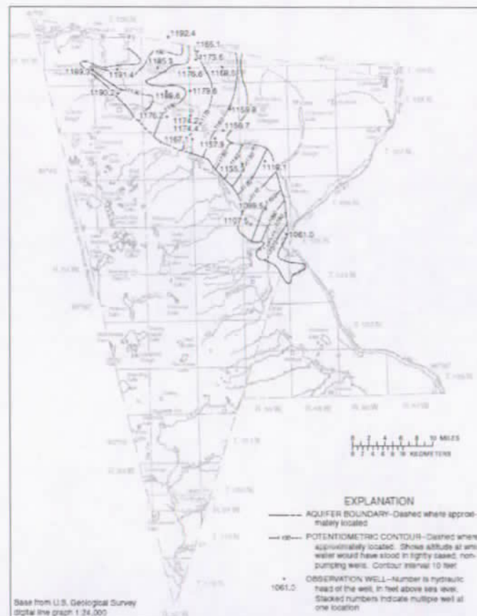
Figure 2- Potentiometric surface of the Veblen aquifer: from Thompson (2001).
