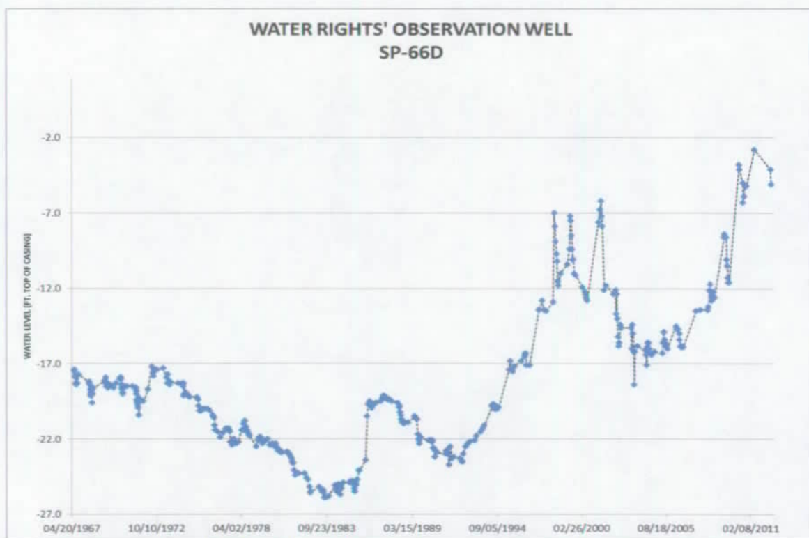
Figure 3. Hydrograph of DENR-Water Rights' observation well SP-66D (see Figure 1 for location)
