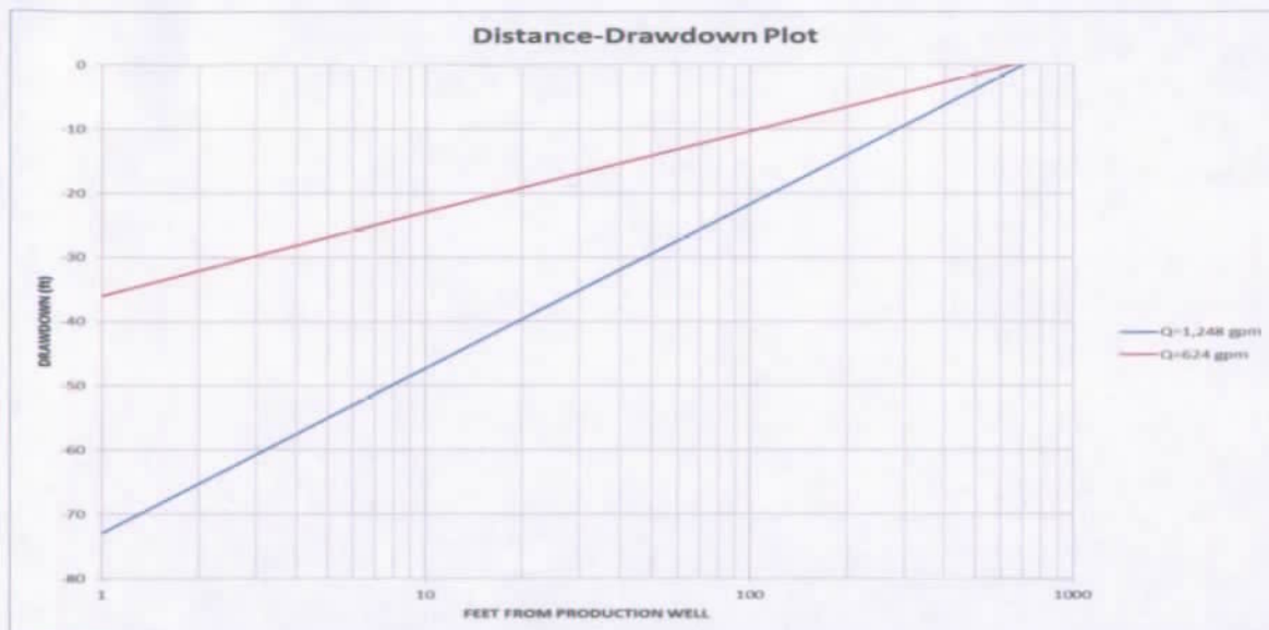
Figure 7. Distance-drawdown plot showing drawdown resulting from a pumping rate of 1,248 gallons per minute using either one well or two wells, and a transmissivity of 25,500 gallons per minute per foot.
