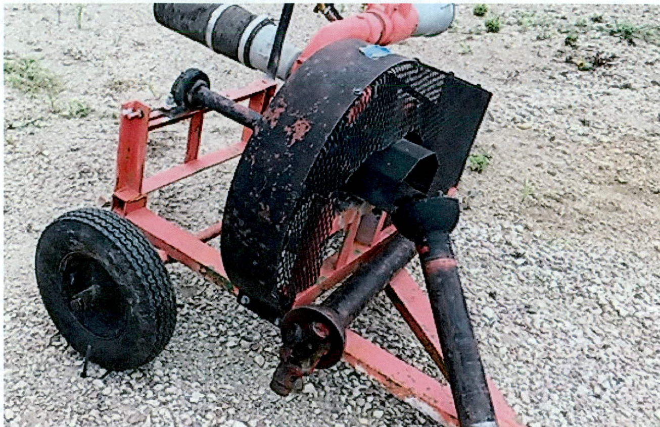
Picture 4. Four inch Berkeley PTO pump. Photo courtesy of Dave Gullickson with Farmers Implement and Irrigation, Brookings SD.
