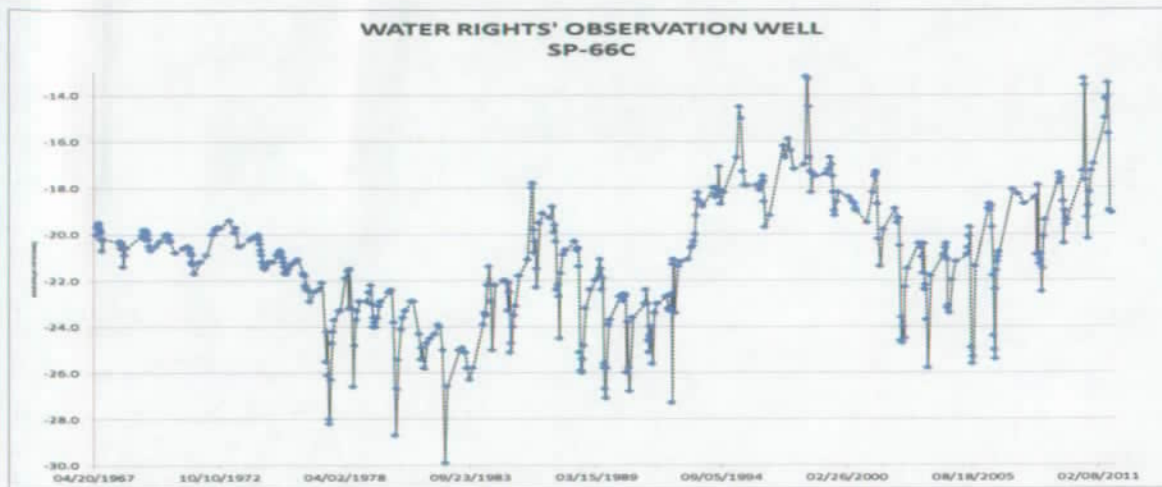
Figure 2. Hydrograph for DENR-Water Rights' Observation Well SP-66C
