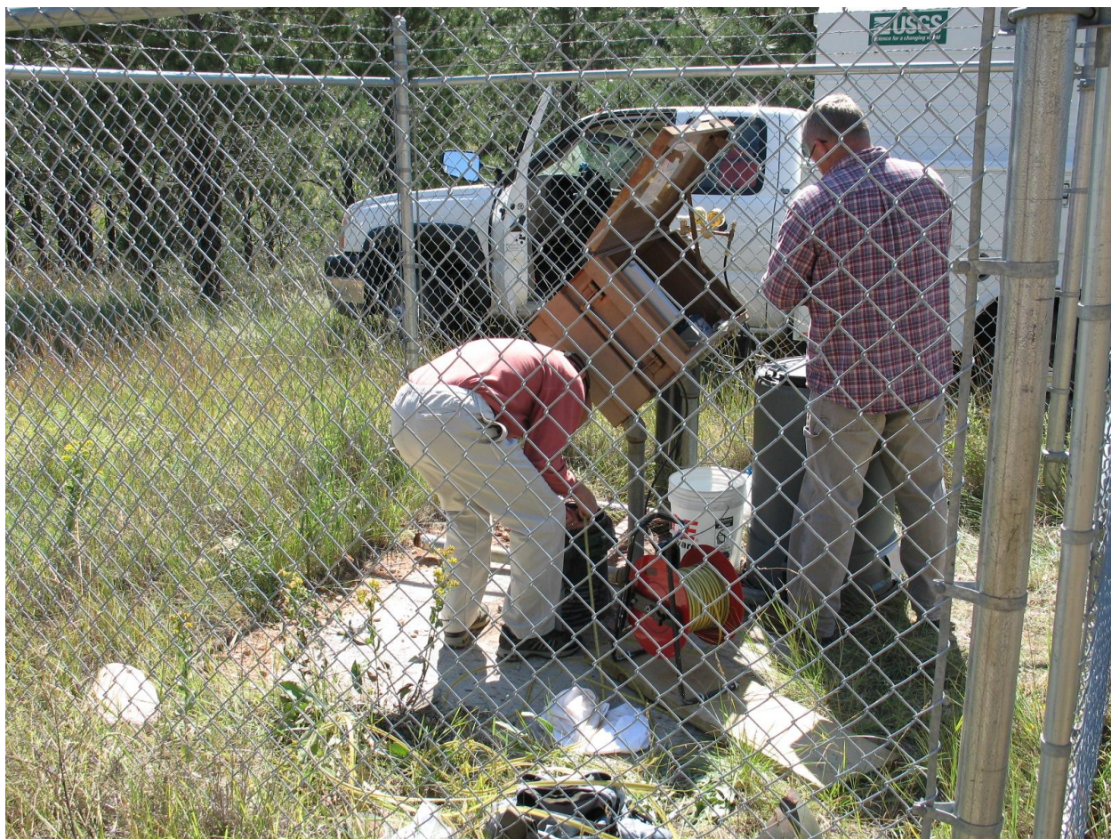
Figure 3. Water level being measured with the electronic well tape in Well No. 2.
