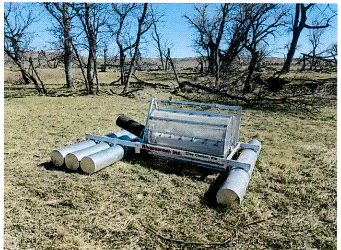
Floating self-cleaning intake screen
