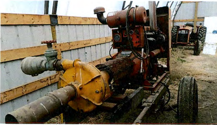
trailer mounted pump
