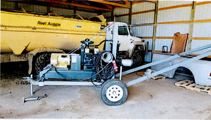
Trailer mounted pump
