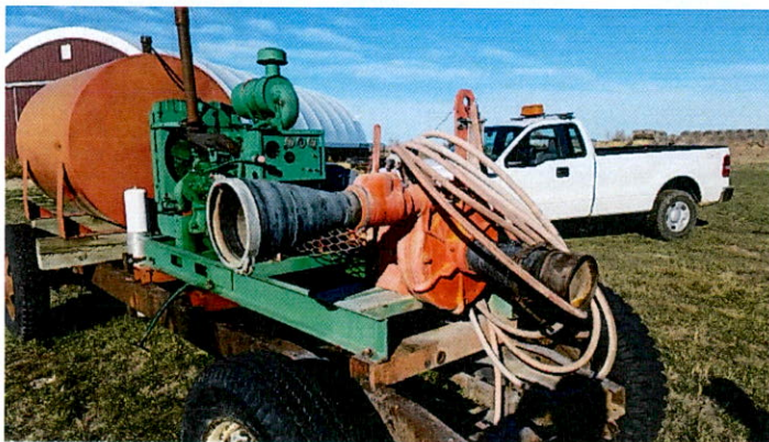
trailer mounted pump
