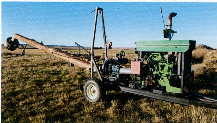
trailer mounted pump
