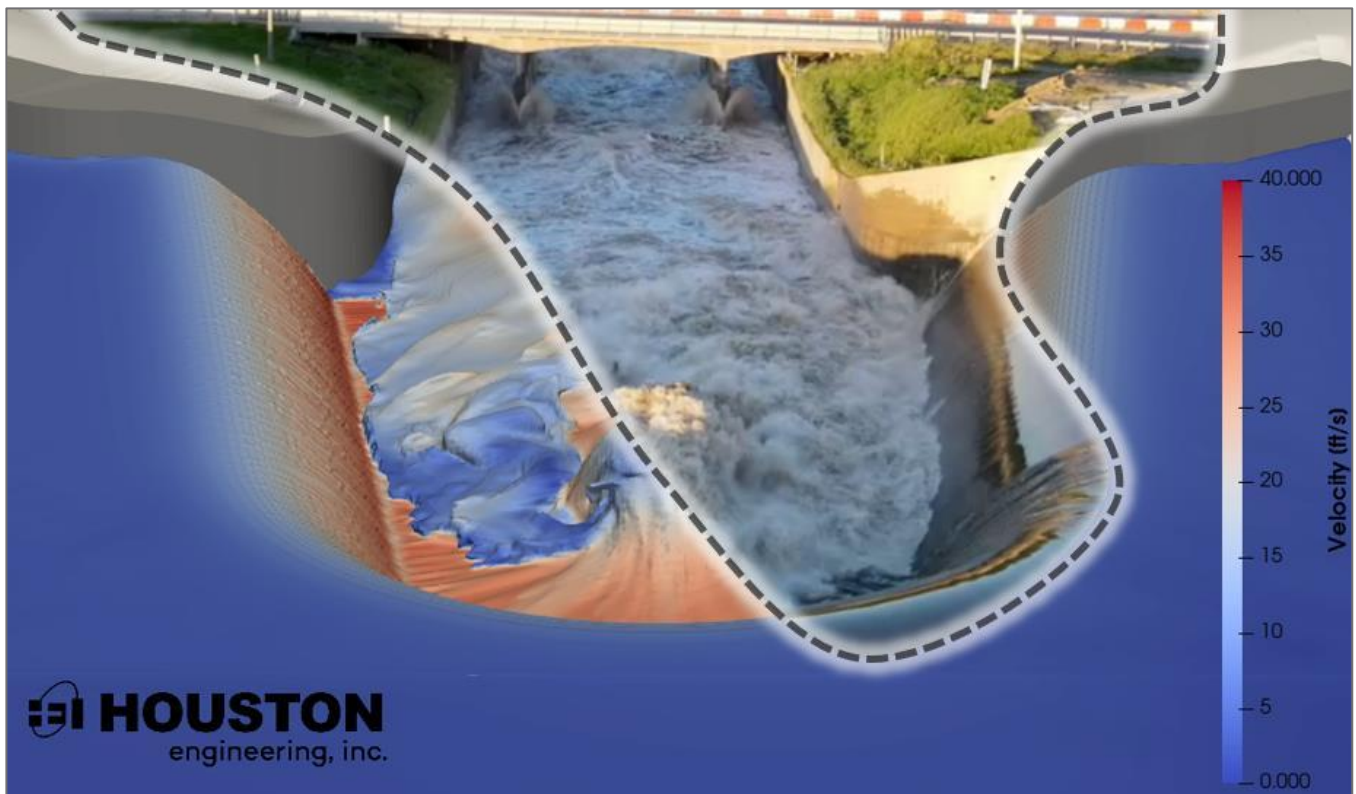
Figure 1 – CFD Modeling matches observed flow patterns within the Lake Mitchell Horseshoe Ogee-weir Spillway
