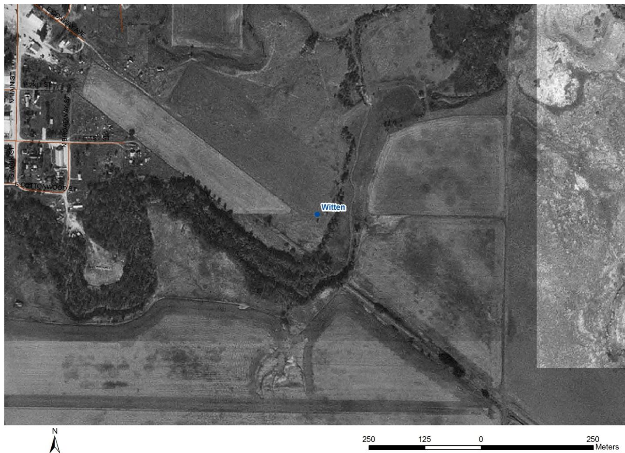
Figure 100. DOQ of Witten dam from 1997. Mature trees and a well-developed channel are visible in the lakebed.
