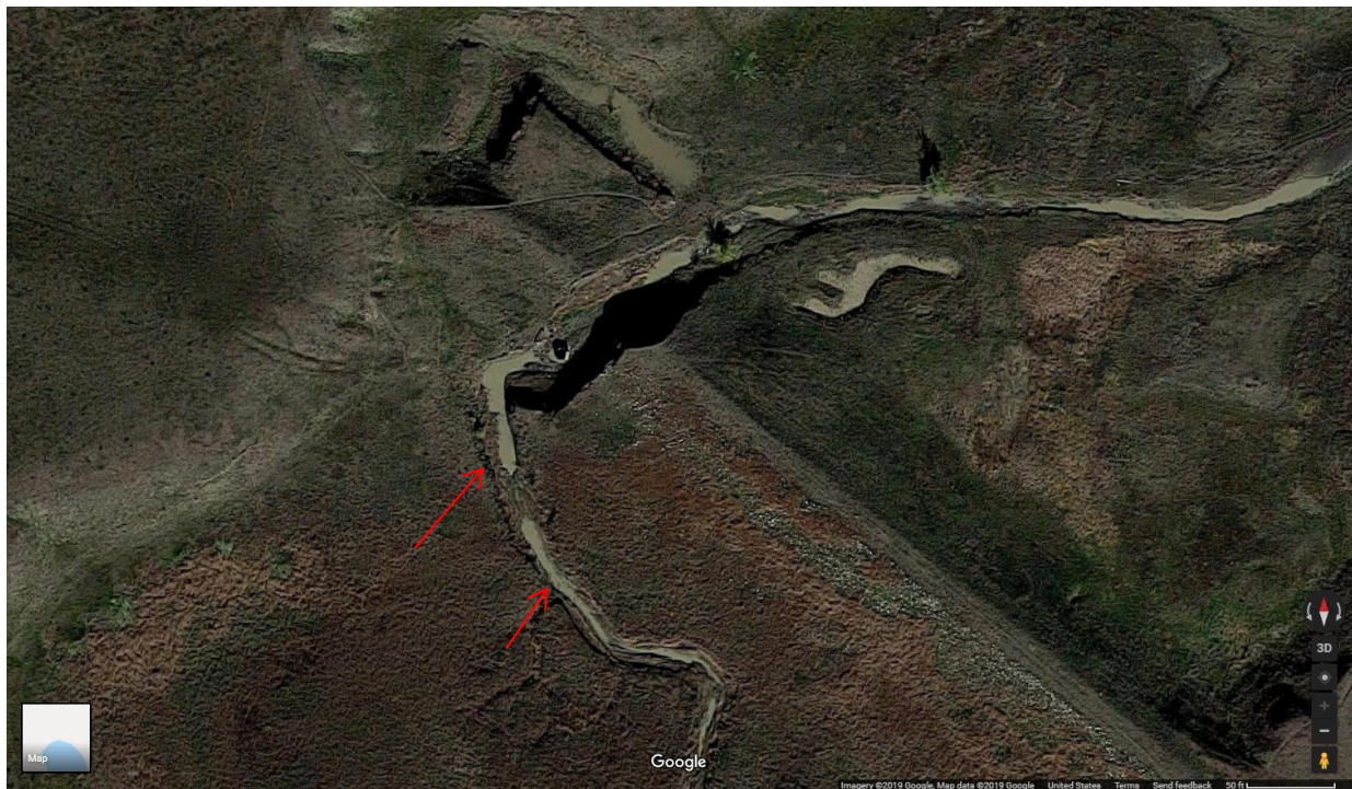
Figure 11. Google image of the Bochart Dam breach and stream channel in the lakebed (red arrows) (Google, 2013).
