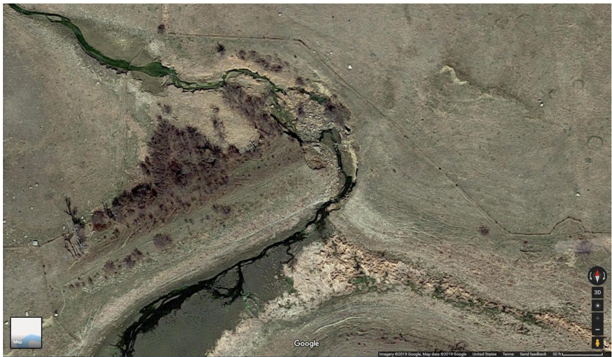
Figure 7. Google Image of Bergers Lake Dam and channel formation through dam grade (Google, 2014)
