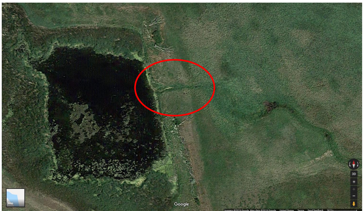
Figure 19. Google Image of Caspers Dam with developing breach visible in red circle (Google, 2016).
