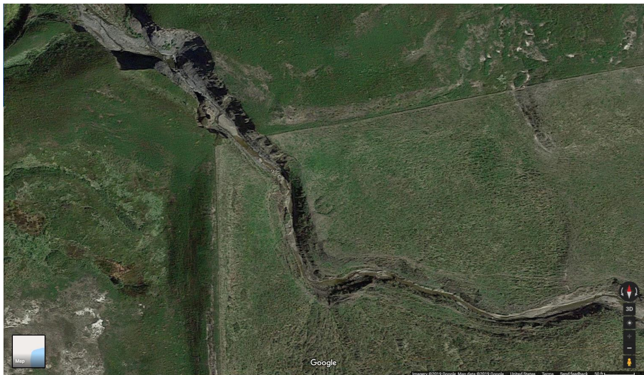
Figure 43. Google image of Goose Creek Dam breach and channel eroded into lakebed (Google, 2014).
