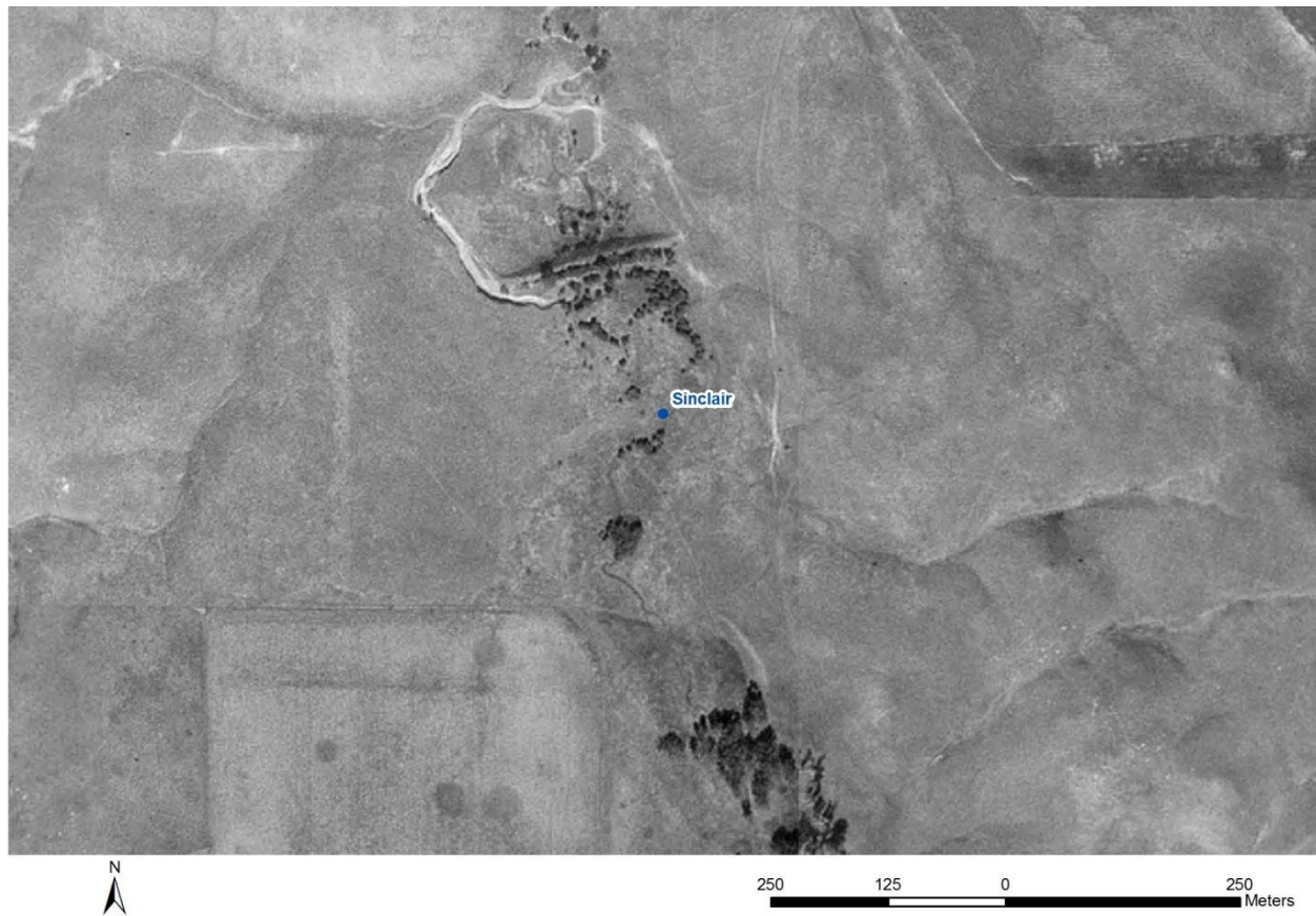
Figure 88. DOQ of Sinclair Dam from 1997 shows a well-developed channel and mature trees in the lakebed.
