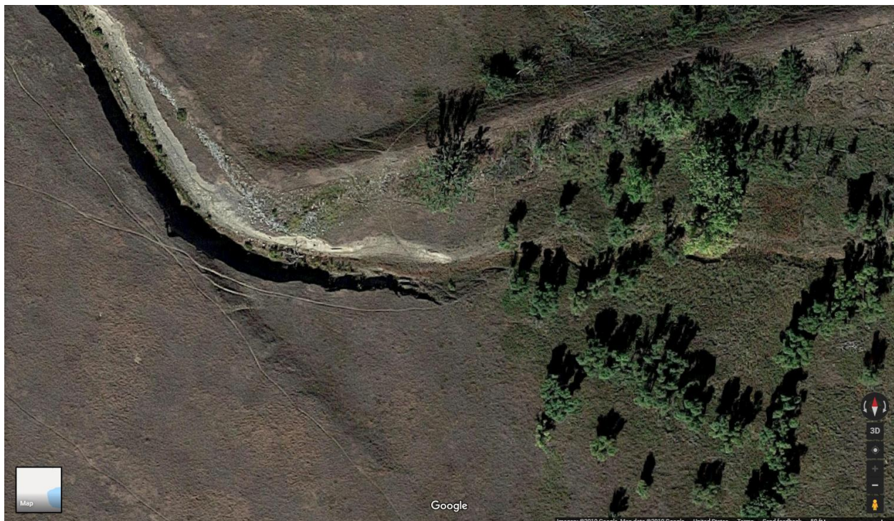
Figure 89. Google image of Sinclair Dam breach with view of mature trees that were present in the 1997 image (Google, 2016).
