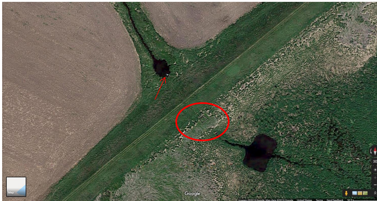
Figure 23. Google Maps Image of the Dam Grade at Cole Lake (Google, 2017). No breach is visible where the stream channel crosses the grade, however a structure, presumed to be a culvert inlet is faintly visible at the center of the circle and the tip of a pipe (arrow) appears at the scour pool to the NW of the red circle.
