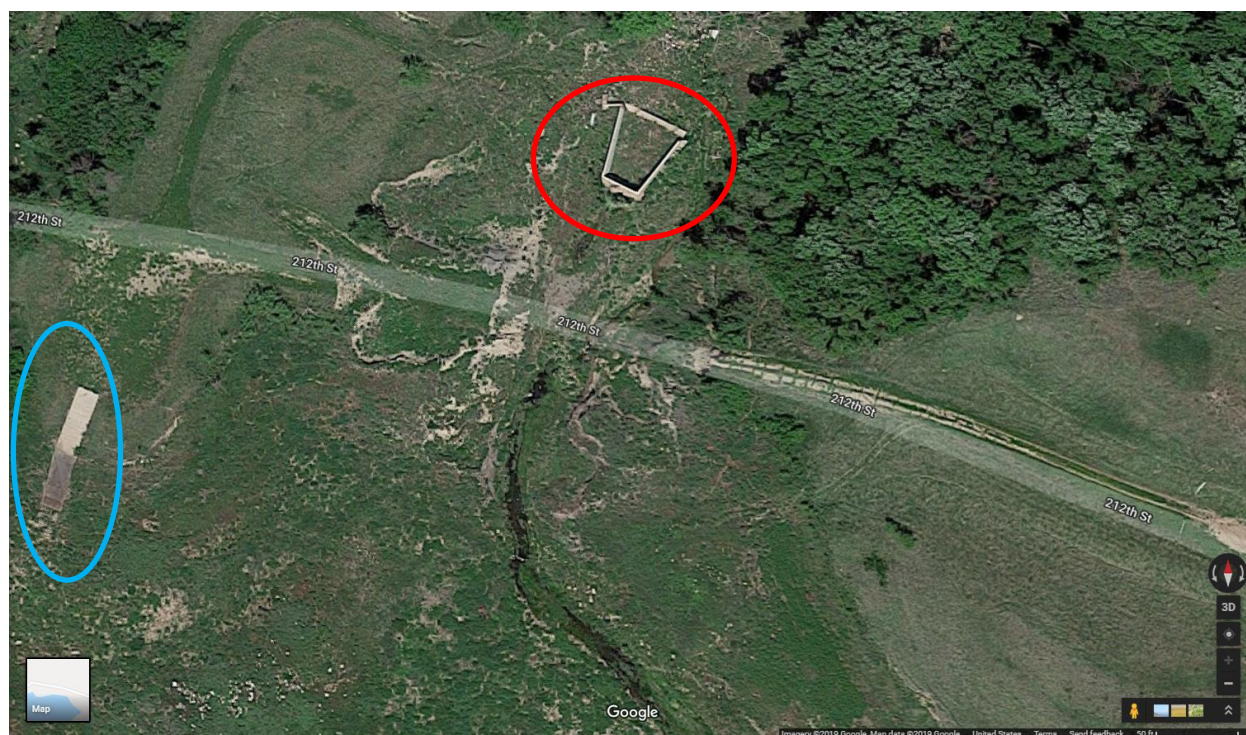
Figure 85. Google image of Rose Hill Dam after most recent breach, out let structure (red circle) and boat ramp (blue circle) are visible (Google, 2014).
