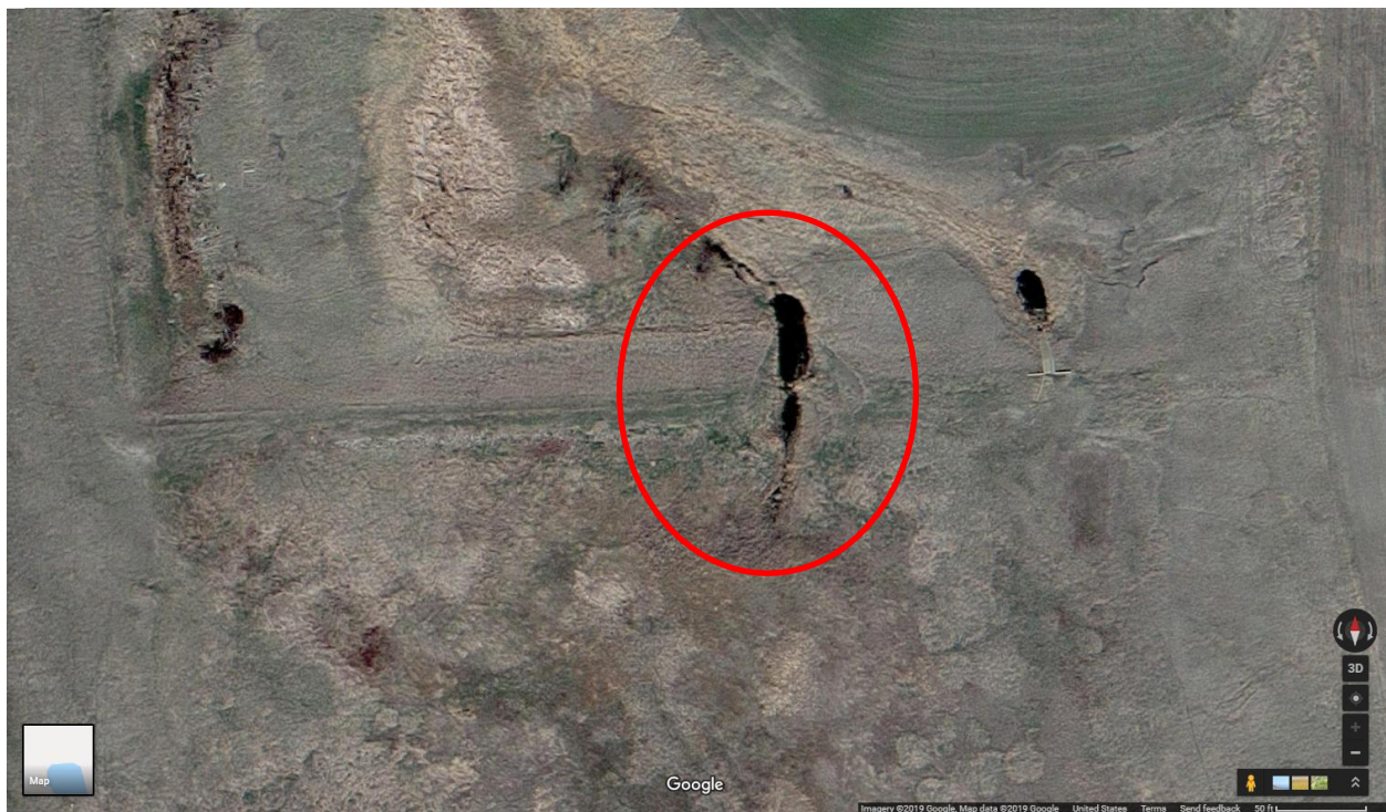
Figure 55. Google image showing the breach in the Kennebec Dam (Google, 2013)
