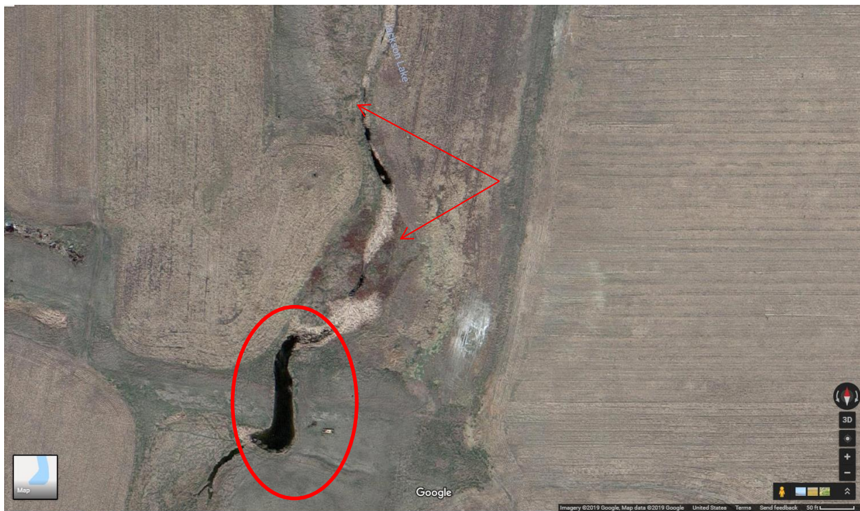
Figure 51. Google image of breach (red circle) in Jackson Dam and developed channel in lakebed (arrows) (Google, 2013).
