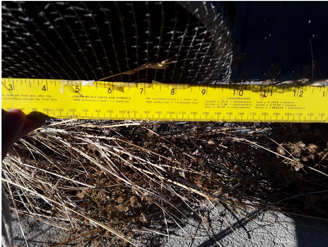
Overflow Screen – Not #24 Mesh
