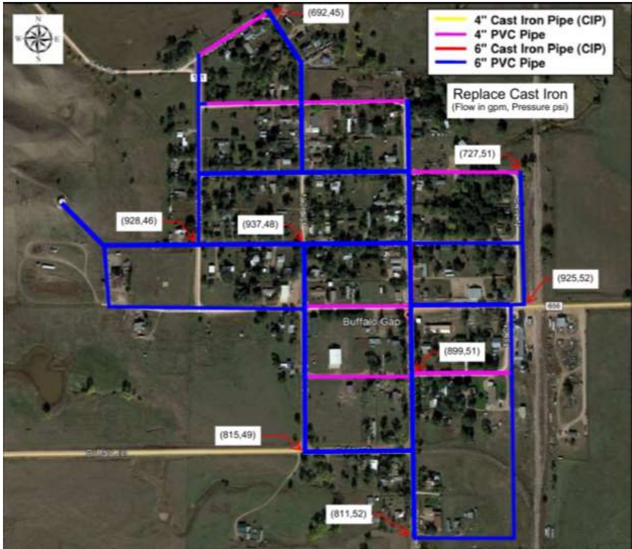
Figure 5.5.2-1: Cast Iron Replacement System Model
