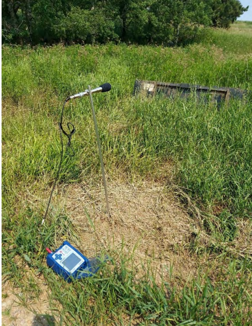
Figure 3-3. Instantel Micromate Sound-Level Meter.
