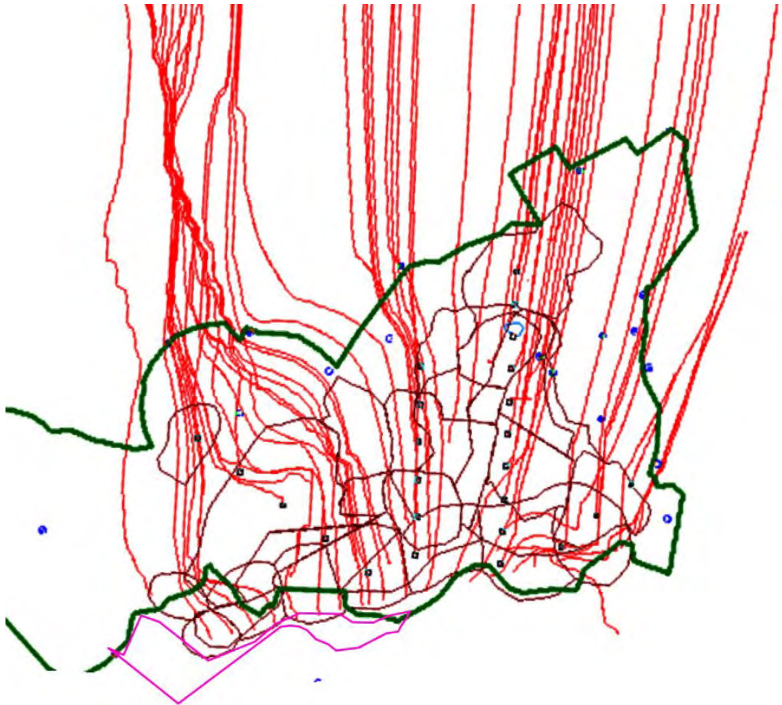
Figure 2-5. Modeled Tracked Particle Flow Lines [Hocking and Minnick, 2019]. Location of the Boston Expansion is approximate.
