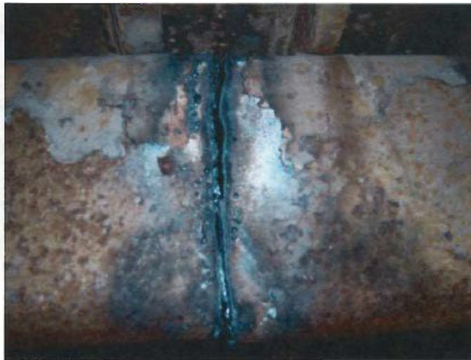
Photo #4: Chassis rail cut in half
