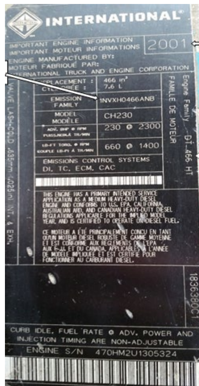
Photo #3: Engine tag with engine serial number and EPA engine family name
