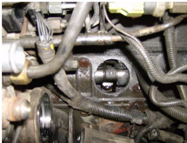
Photo #6: Engine block after hole has been drilled
