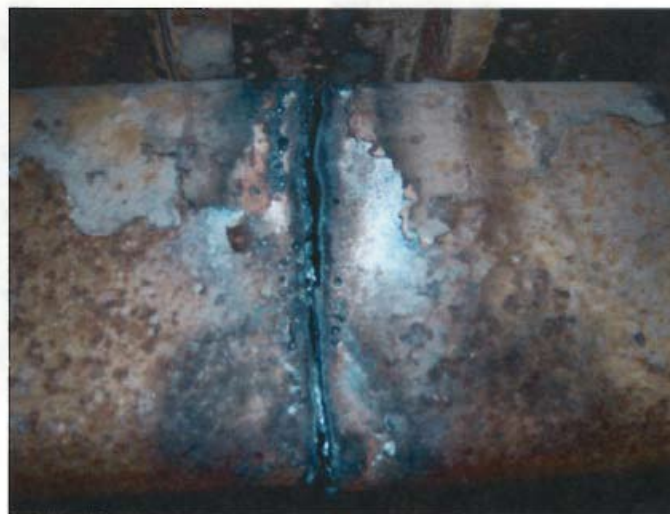
Photo #4: Chassis rail cut in half
