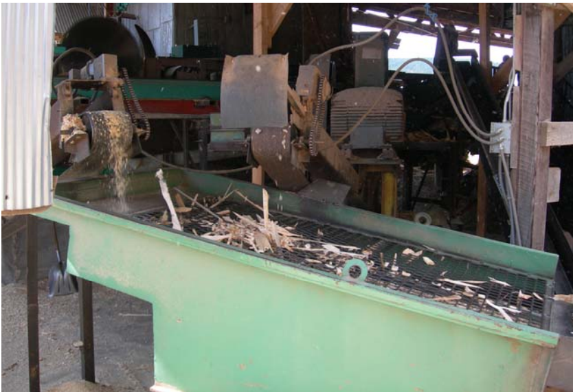
Photo 12 – Sizing equipment used for removing over-sized chips and fines at the Sturgis Sawmill.
