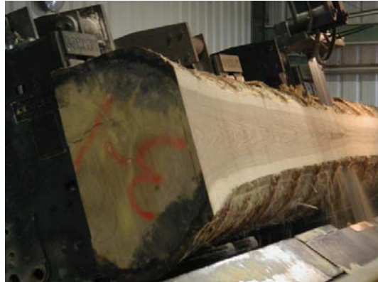
Photo 3 - A debarked log being cut into dimensional lumber.
