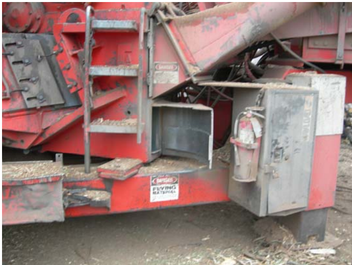
Photo 10 – Fines separator/discharge feature on a Morbark whole-tree chipper.
