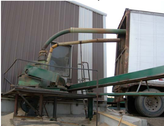
Photo 4 -Chips and sawdust being blown directly into a live bottom trailer at a post and pole mill.
