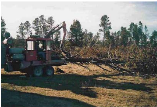
Photo 8 – Whole trees chipped into heating fuel in Chadron, Nebraska. (Photo courtesy of Tom Coston, Bitterroot RC&D)
