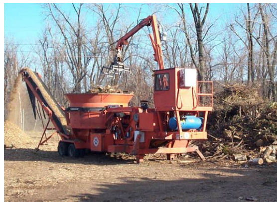
Photo 5 - Community wood trimmings being ground into chips using a tub style grinder.
