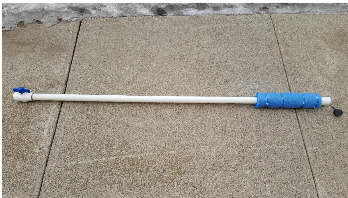
Figure 3. Photo of integrated depth sampler for lakes.
