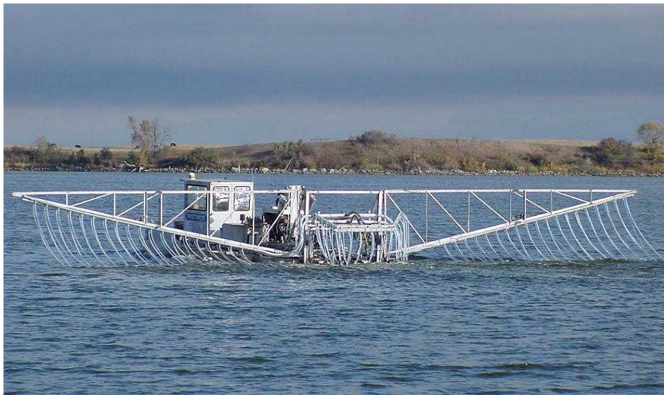
Barge Applying Alum to Lake Oliver to Reduce Inlake Phosphorus (Cochrane/Oliver Watershed)
