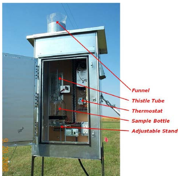
Figure 13. Typical construction of a passive bulk mercury atmospheric sampler
