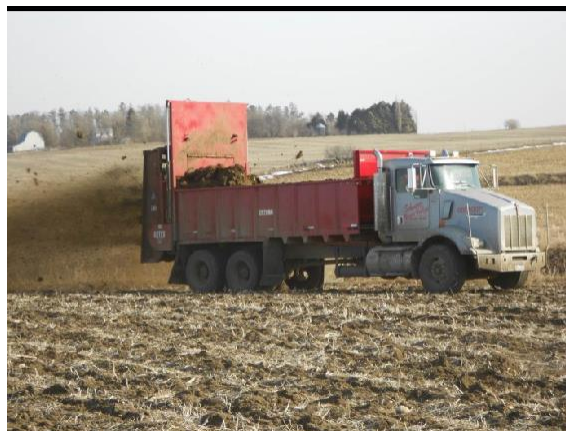
Figure 3. Application truck with vertical beaters, 2014.
