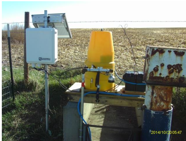
Figure 4. Automated monitoring and sampling equipment installed in late 2014. Shown are the automated sampler (yellow), battery (black box), ultrasonic depth sensor (in front of automated sampler), and data logger in the new white enclosure. A solar panel is mounted on the pole on the far side of the data logger enclosure. The white box on the right in the foreground formerly housed the Stevens stage recorder.
