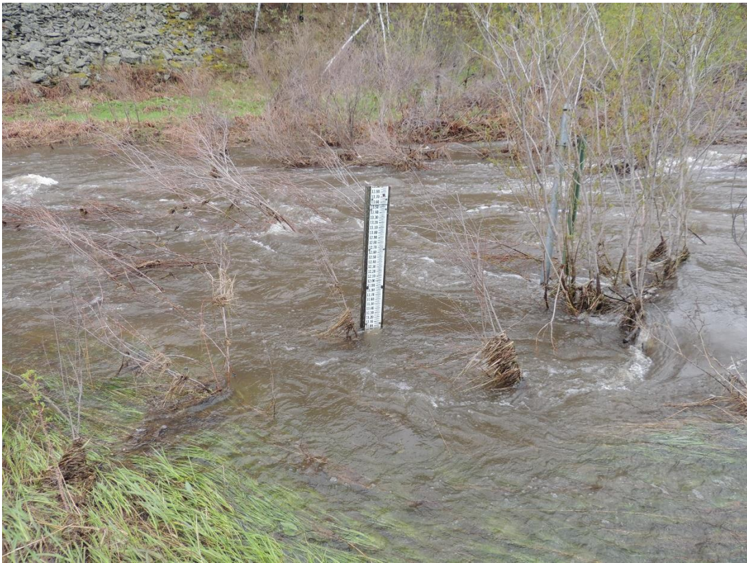
Figure 22. Staff gage at inlet to Sheridan Lake, May 28, 2015
