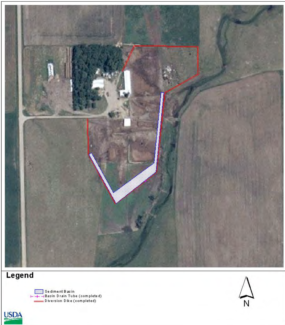
Figure 2. Clean Water Diversion System.
