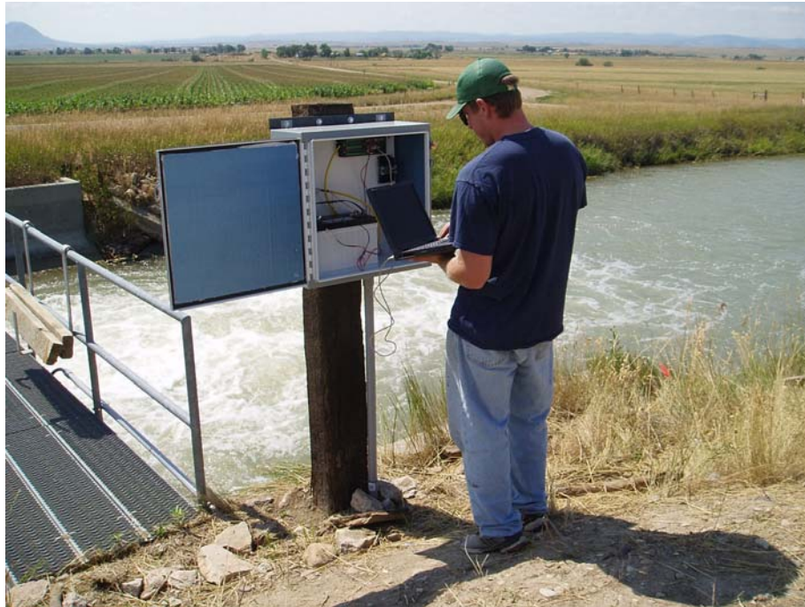
Figure 7. Data Collection From Flow Automation Unit Used for Canal Operational Model.
