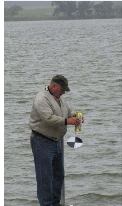
Monitor Taking a Secchi Disk Reading on Oakwood Lakes.
