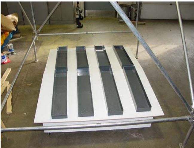
Figure 4. Runoff boxes used for indoor rainfall simulation.
