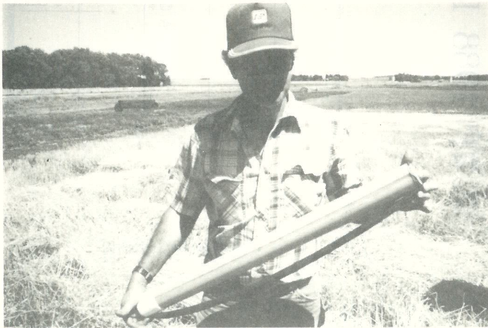
Figure 3-9. A stainless steel porous water sampler with a rubber tube located beneath to force the unit to contact the soil after lateral insertion.
