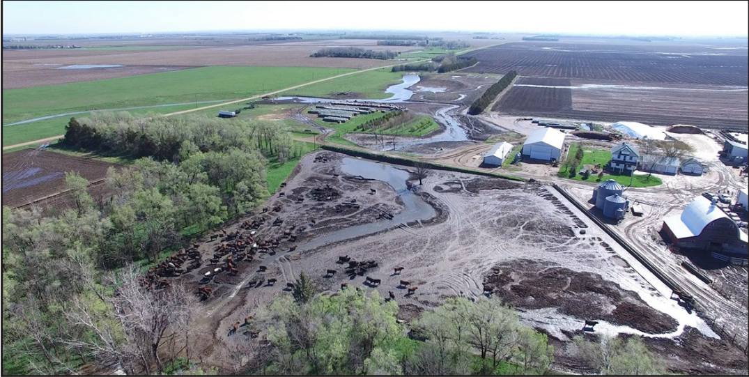
Figure 44, 45, 46 .Photos from feedlot prior to construction, site was on a creek that when flooded would flood the feedlot pens.
