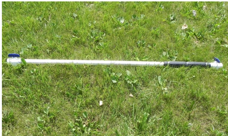
Figure 3.0. 2 Modified integrated depth sampler based on MPCA Sampler.
