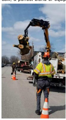
large tree at almost lightning speed! Plus, since the operator is guiding the entire operation with a joy-stick, they have significantly reduced their exposure to the many hazards of tree removal.
