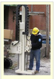
A geoprobe is used to collect a soil sample at an old hospital property. Phase II sampling can determine whether a release has occurred, delineate the extent of the contamination, develop a cleanup cost estimate and determine a baseline environmental condition for liability purposes.
